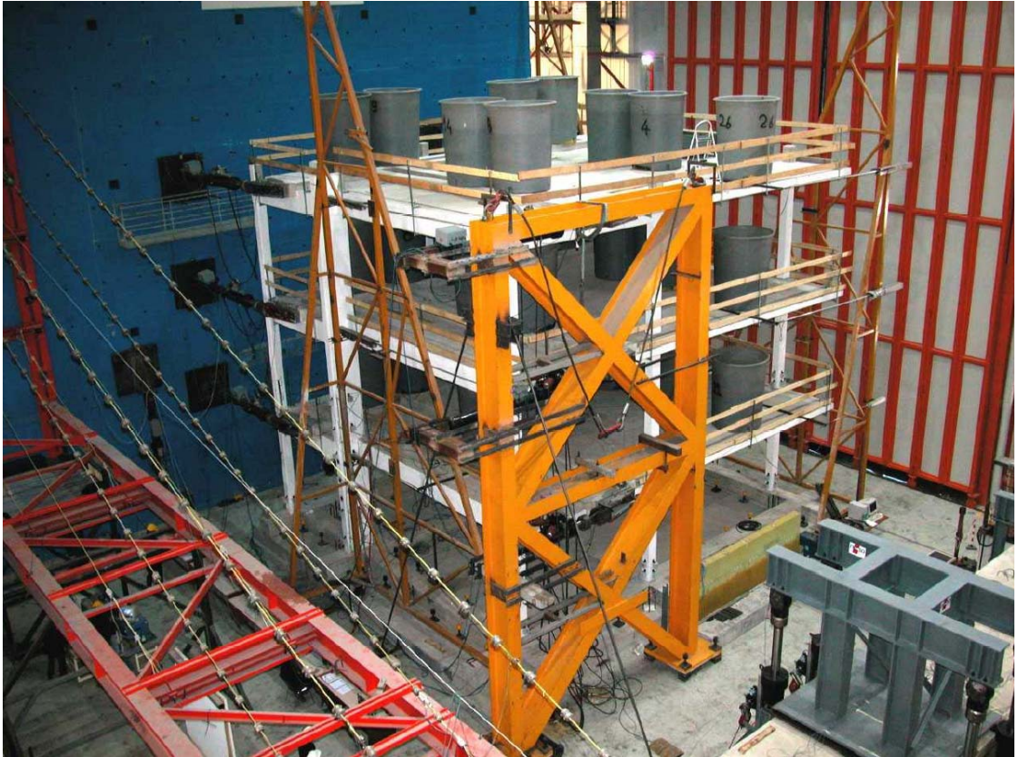
Fig. 2. View of the SPEAR structure ready for the bidirectional PsD tests
